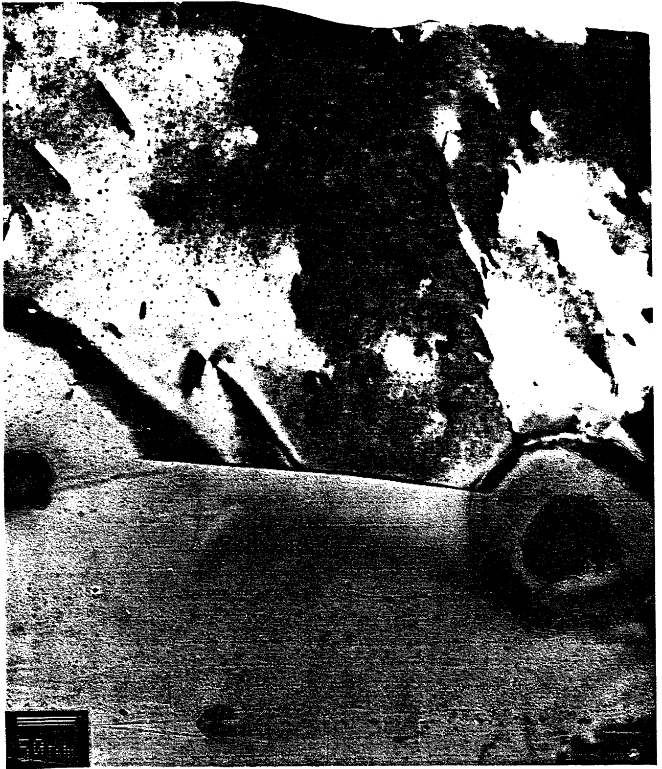
FIGURE 2. Microstructure of As-Received MA957 Bar Showing a Longitudinal Section Using Transmission Electron Microscopy at 300,000x.
