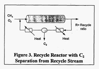
Experimental results using a recycle reactor have been reported recently by Vayenas and coworkers. Their reactor had a per-pass methane conversion of less than 3%. However, at steady-state, they report a maximum  $C_2$  yield of 49%, at a  $CH_4$  conversion of 65%. Furthermore, in batch operation ( $R = \infty$ ), the reactor achieved a  $C_2$  yield of 88%, the highest value reported to date for the oxidative coupling reaction. As
