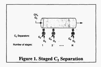
increases, the overall reactor performance (and complexity) also increases. Fortunately, a small number of separators (<10) gives a significant improvement in  $C_2$  yield. The maximum  $C_2$  yield ( $N = \infty$ ) is about 90%, corresponding to the selectivity of the surface methane oxidation reaction.
