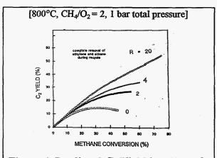
Figure 4. Predicted C<sub>2</sub> Yield in a Recycle Reactor with Increasing Recycle Ratio
