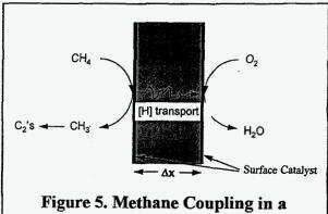
Hydrogen Transport Membrane Reactor
