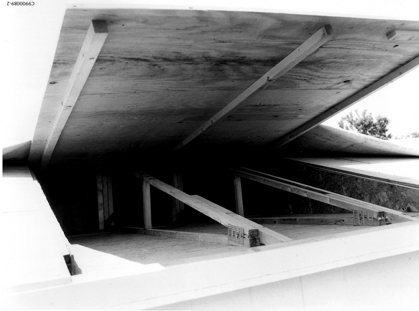
Figure 4. Photograph of roof test facility with one test section open.
