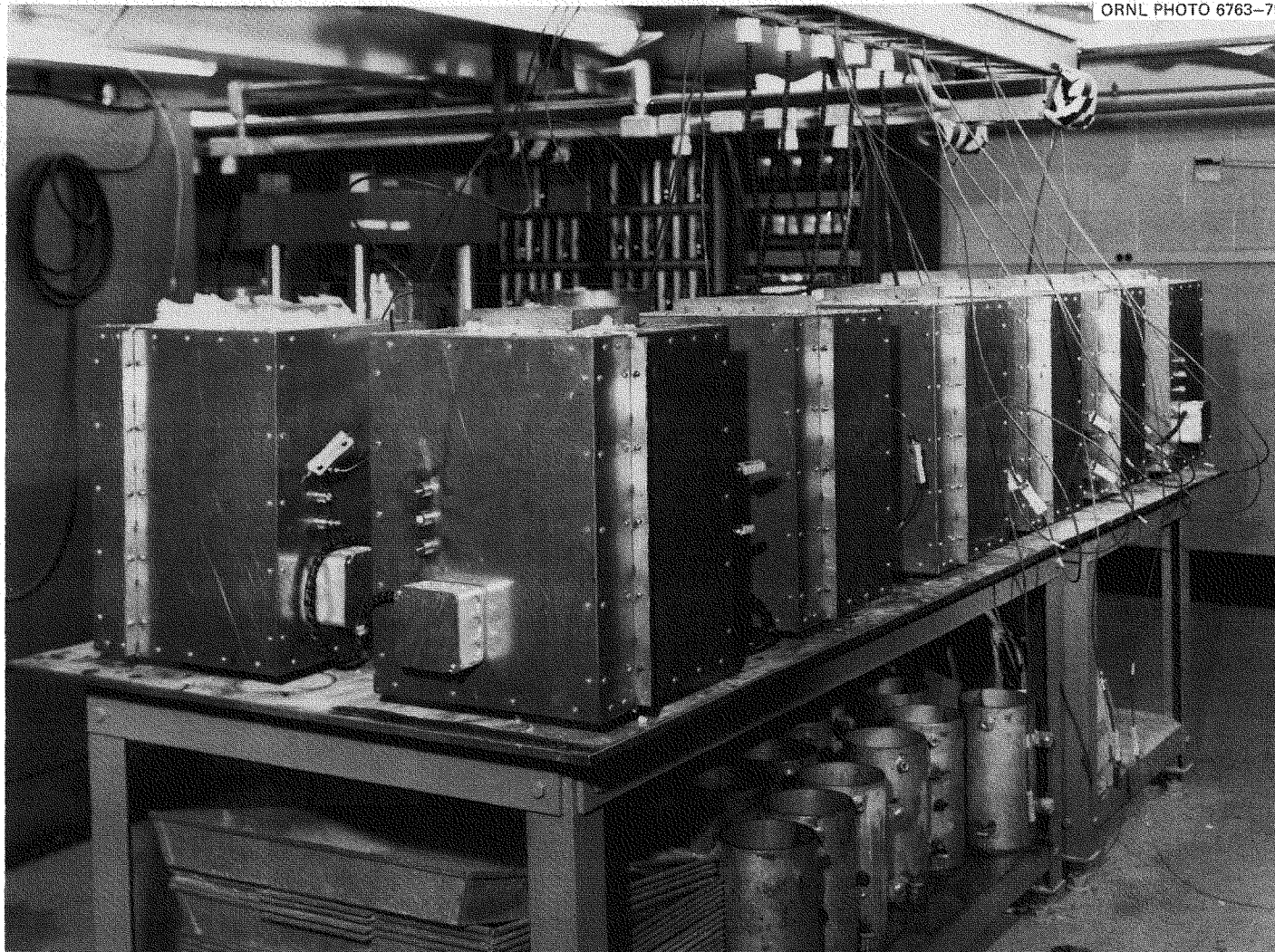
Fig. 8. Shear test furnaces during heat-up.
