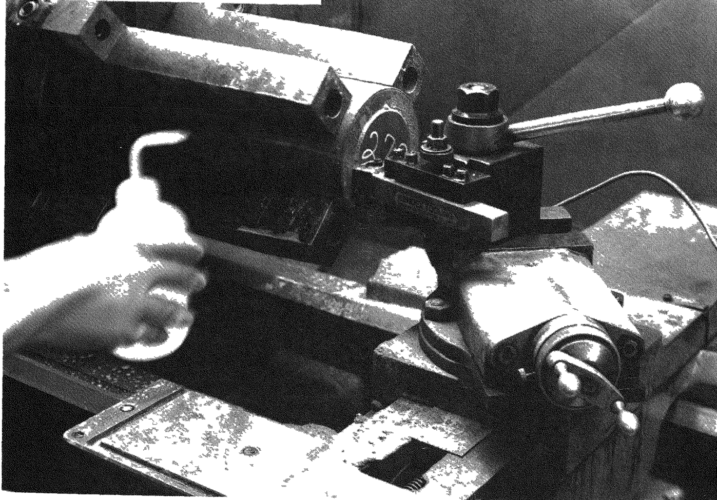
Fig. 3. Machining compression and sustained load test specimens.
