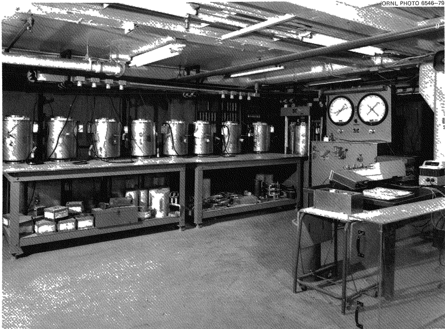
Fig. 5. Compression test furnaces during heat-up.
