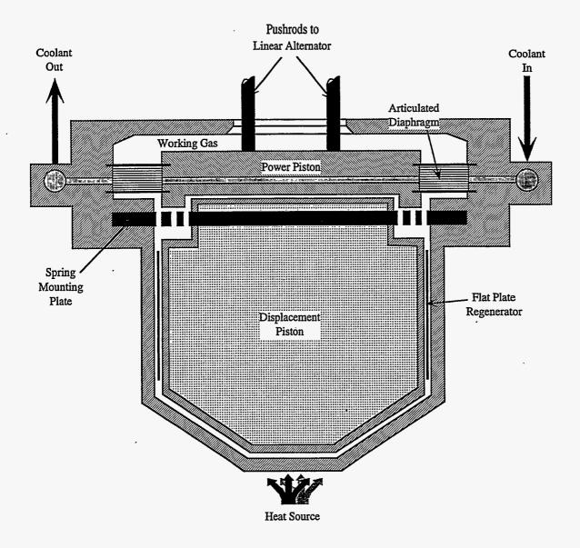
Figure 4—Stirling Engine
