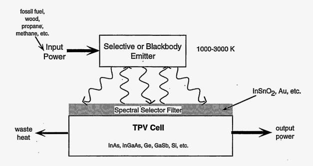
Figure 3—Thermophotovoltaic System Concept
