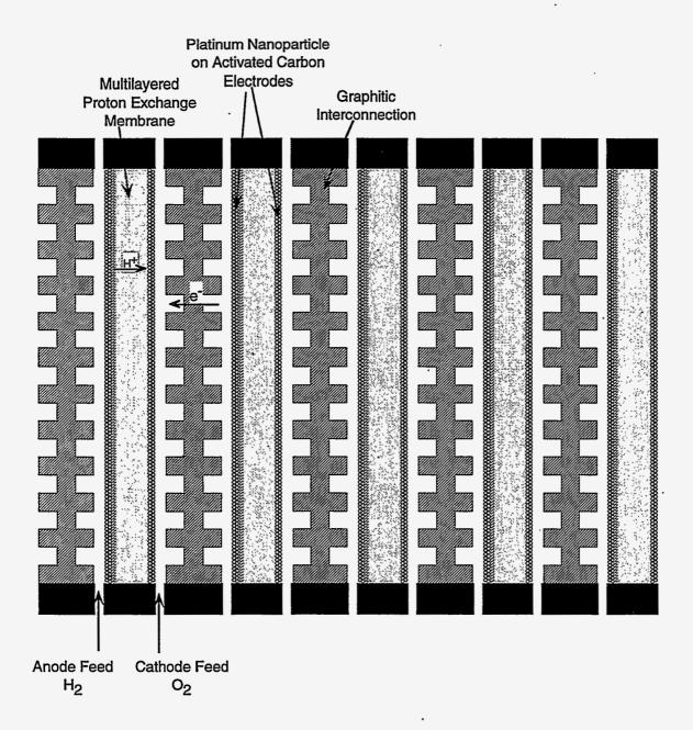
Figure 2—Fuel Cell Stack Cross Section
