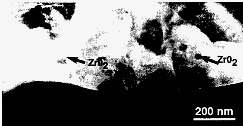
Fig. 8. Annular dark-field STEM image of cross-section through scale showing \text{ZrO}_2 particles within the scale.
