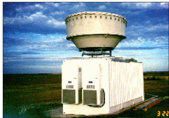
Figure 2. The millimeter-wave cloud radar (MMCR) located at the ARM SGP central facility.
