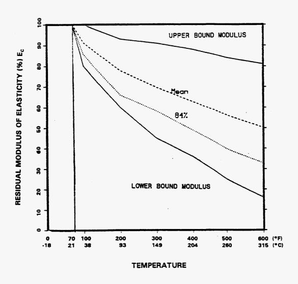
Figure 2 Variation of the Modulus of Elasticity of Concrete with Temperature
