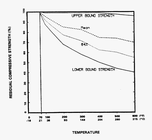
Figure 1 Reduction of Compressive Strength of Concrete at Elevated Temperature
