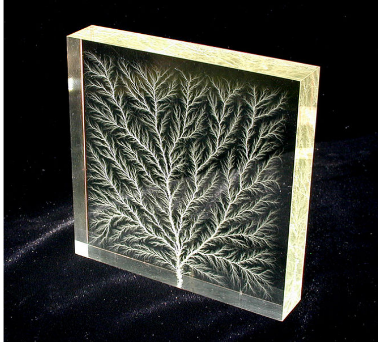
Figure 3.4 Plexiglas after breakdown voltage limit was applied and reached.
