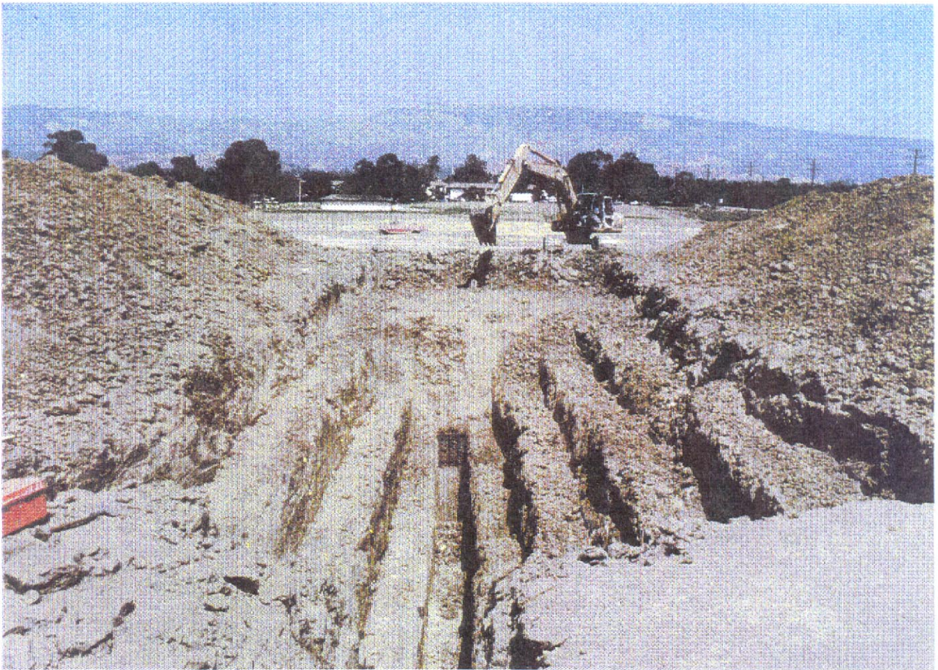
Figure 21. (top) Trench excavated across More Ranch fault to evaluate slip rates
