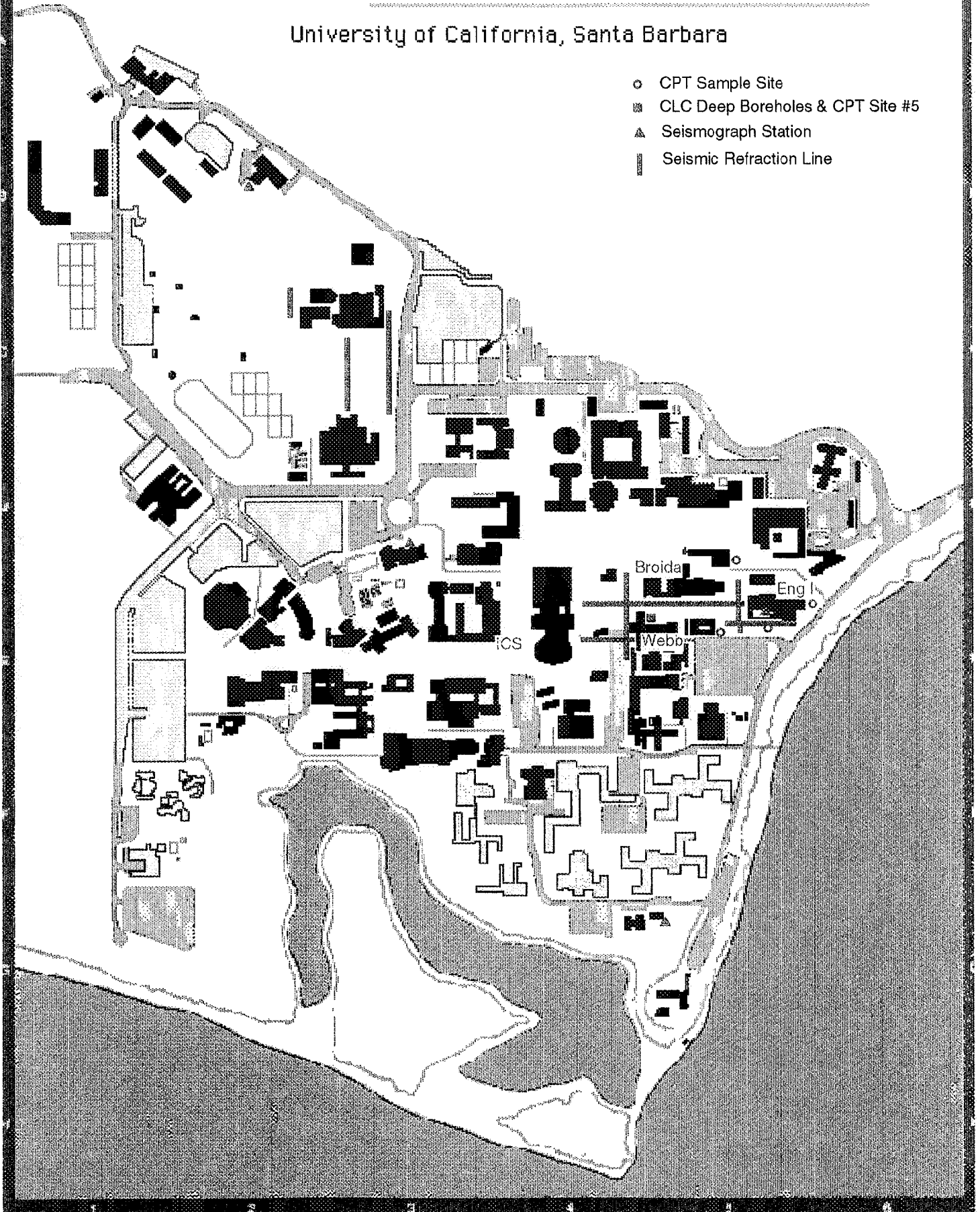
Figure 4. UC Santa Barbara campus showing locations of Engineering I, Broida, Webb, seismic refraction profiles (red lines), seismic stations (triangles), CPT sites (circles), and the CLC deep drill site (square).
