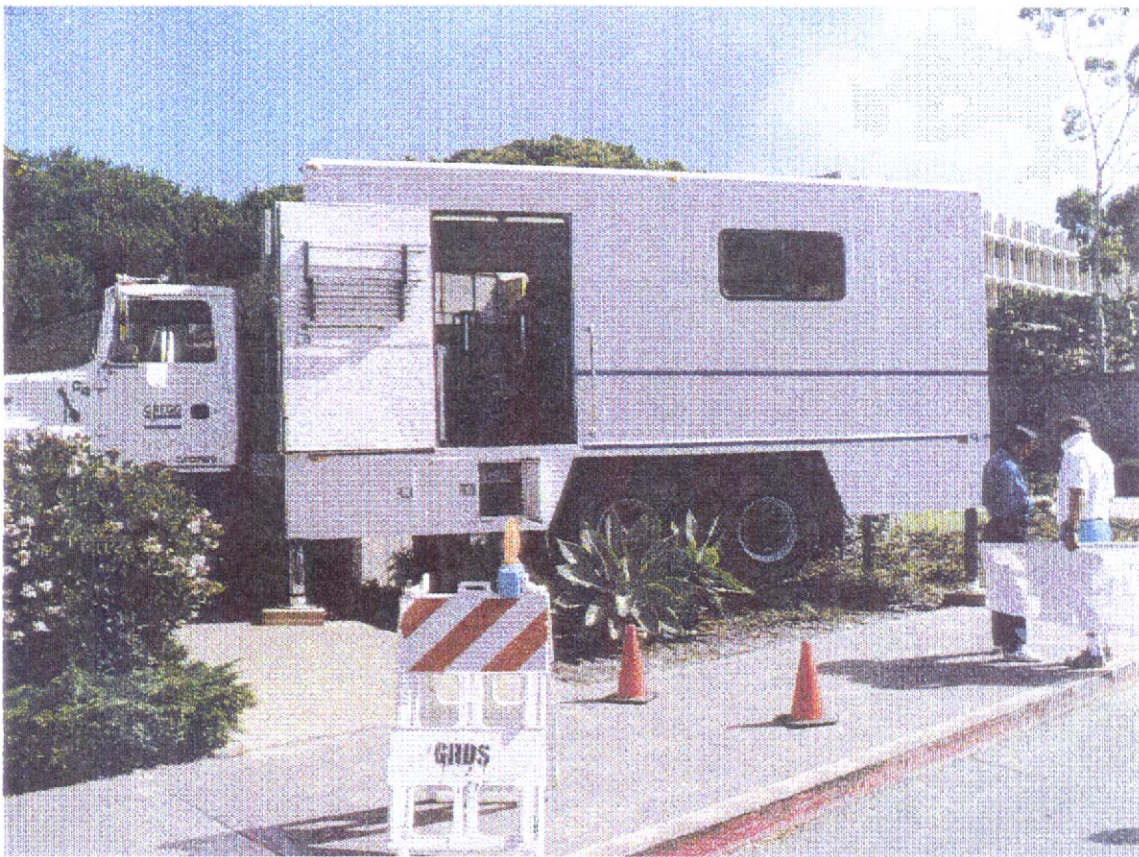
Figure 24. (top) Cone-penetration test (CPT) truck in operation at UCSB adjacent to Woodhouse Laboratory.
