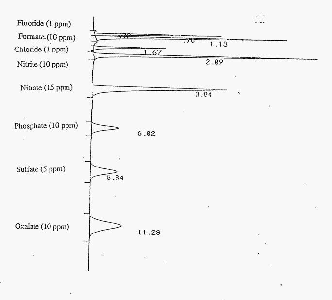
detector range = 30 uSintegrator attenuation = 1024
