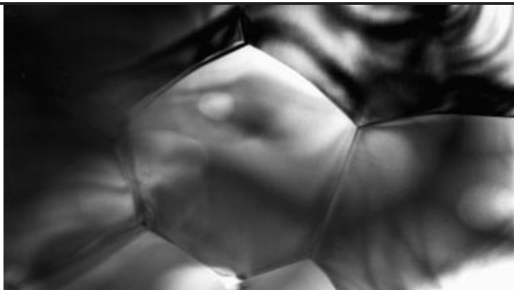
Figure 1. The grain structure of the 99%-dense sample, revealing equilibrated, hexagonal-shaped grains with sharp apexes, with a mean grain size of about 4 \mu\text{m} .
