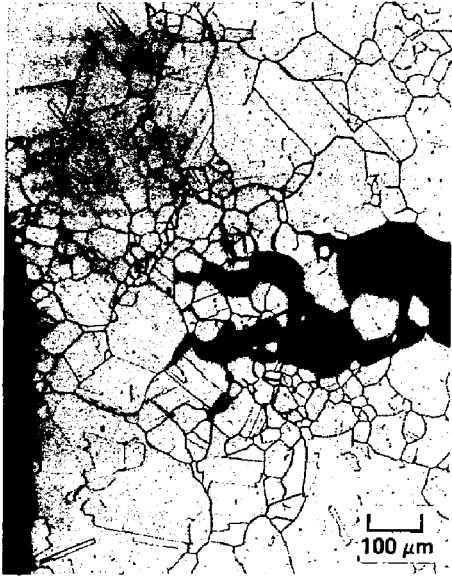
Figure 4. Metallographic cross sections of sensitized Type 304 U-bend specimens showing IGSCC. Source: Juhas et al. (1984) and Westerman et al. (1987).
