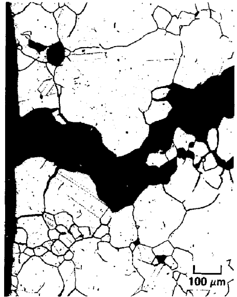
Figure 4. Metallographic cross sections of sensitized Type 304 U-bend specimens showing IGSCC. Source: Juhas et al. (1984) and Westerman et al. (1987).
