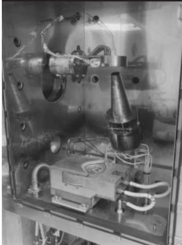
Figure 1: Photograph of apparatus used for NBAD of BN films.
