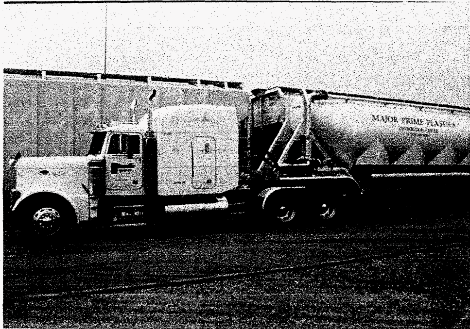
Figure 4.4 Side view of a pneumatic dry bulk transport tank loading from a pressure differential rail car
