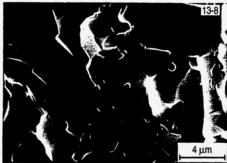
Figure 16. Fracture surfaces of 12-5 and 13-8 samples sintered at 1600°C for 300 min.
