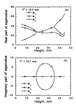
Fig. 3. Eigenvalues of maglev system vs. vehicle levitation height with  $Y^* = 12.7 \text{ mm}$
