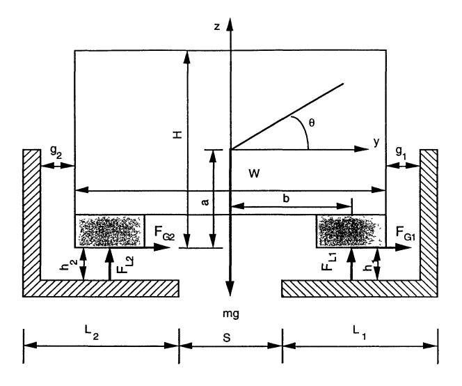
Fig. 2. Maglev system with a vehicle on a double L-shaped aluminum sheet guideway
