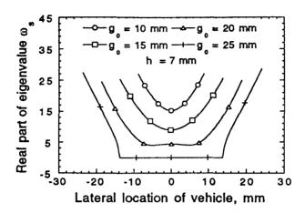
Fig. 5. Real part of eigenvalues of maglev system vs. lateral location of vehicle with h = 7 mm and  $g_0 = 10$ , 15, 20, and 25 mm
