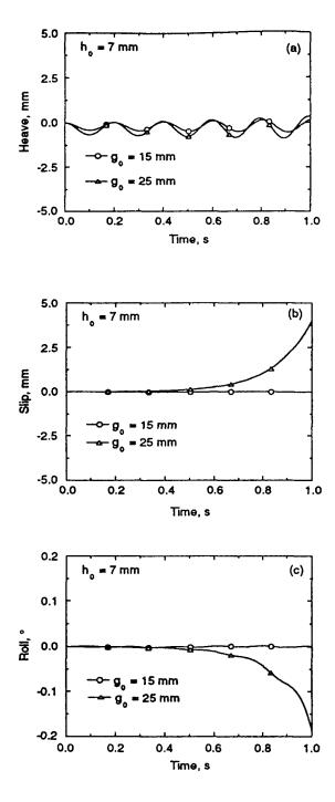
Fig. 7. Time histories of vehicle motions with various lateral air gaps  $g_0$  when  $h_0 = 7$  mm.
