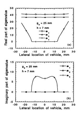
Fig. 4. Eigenvalues of maglev system vs. lateral location of vehicle with h = 7 mm and  $g_0 = 25$  mm
