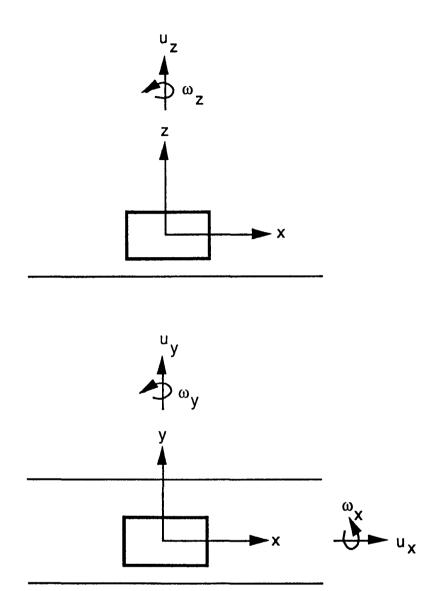
Fig. 1. Displacement components of a maglev system
