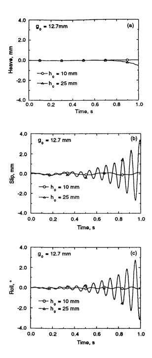
Fig. 6. Time histories of vehicle motions with various vertical air gaps  $h_0$  when  $g_0 = 12.7$  mm.
