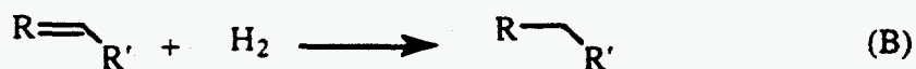
Figure 3.2 Non-free radical reaction families included in NBBM model: (A) naphthyl hydrogenation; (B) olefin hydrogenation.
