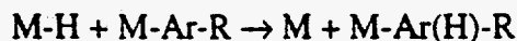
Figure 5.7 Chemical equation for an ipso insertion of a catalytically bound hydrogen atom to an aromatic ring.
