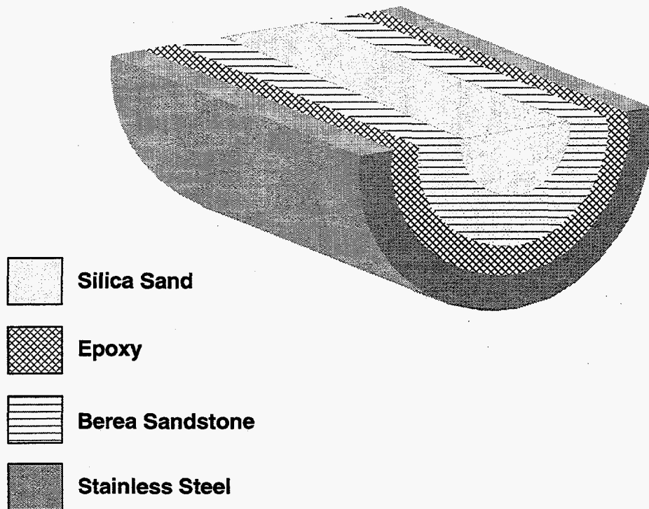
Fig. 11. Mobility dependence on permeability in a series composite core #2.
