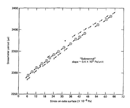
FIG. 2b. "Subnormal" calibrations for laboratory tests in granite cube.
