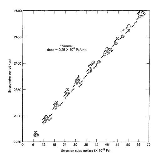
FIG. 2a."Mcrmal" calibrations for laboratory tests in granite cube.
