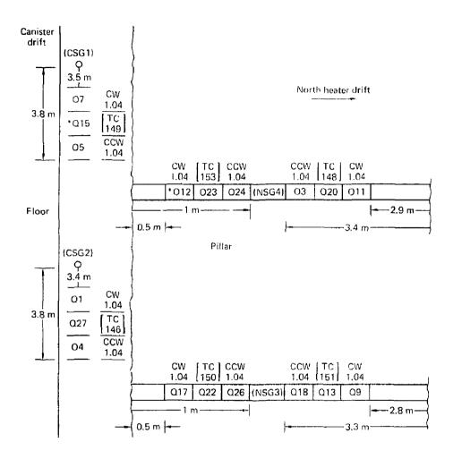
FIG. 5. Stressmeter placements (CW, clockwise; CCW, counterclockwise; TC, thermocouple; also, hole designations are given in parentheses).
