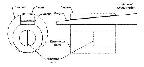
FIG. 1. Schematic of stressmeter in borehole.
