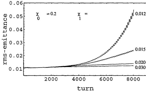
FIG. 2. Multi-particle simulation result showing stabilization of the HT motions of the rms-emittance of a Gaussian beam when  $\chi_1 \geq 0.026$  - the theoretical stability threshold of the  $l = 1$  mode [cf. Eq. (11)]. Here  $\chi_0 = 0.2$ ,  $\Upsilon = 0.22$ .
