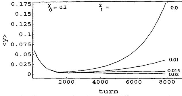
FIG. 1. Multi-particle simulation results showing stabilization of the HT motions of the centroid of a Gaussian beam by  $\chi_1$ , where  $\chi_0 = 0.2$ ,  $\Upsilon = 0.22$ . The estimated stability threshold for the  $l = 1$  mode, according to Eq. (8), is where  $\chi_1 \geq 0.0127$ .
