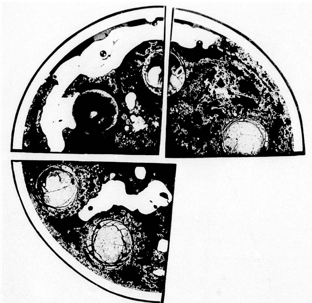
Fig. 49. Transverse Section through Fuel Region about 1.6 cm below Original Top of Fuel Columns. Sections 147A39L and 147A46R. Neg. No. MSD-185659.
