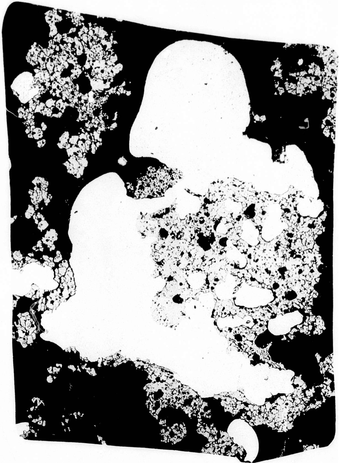
Fig. 50. Melted Steel in Melted Fuel. Section 147A39L. Mag. 85X. Neg. No. MSD-158400.
