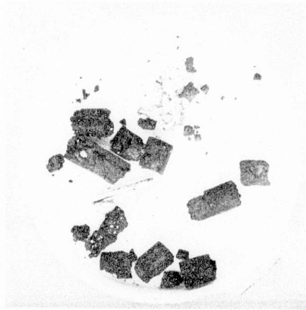
Fig. 34. Fuel section from 147A13, 147A14, and 147A15. Fuel is 70% UO 2 , 20% Na 2 CO 3 , and 10% Na 2 O.
