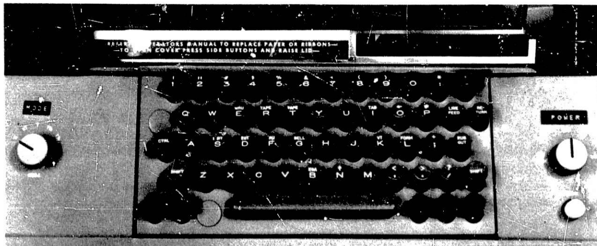
Fig. 48. Teletype (ASR 35) Used to Input Commands and Print Out Data. ANL Neg. No. 103-R5719.
