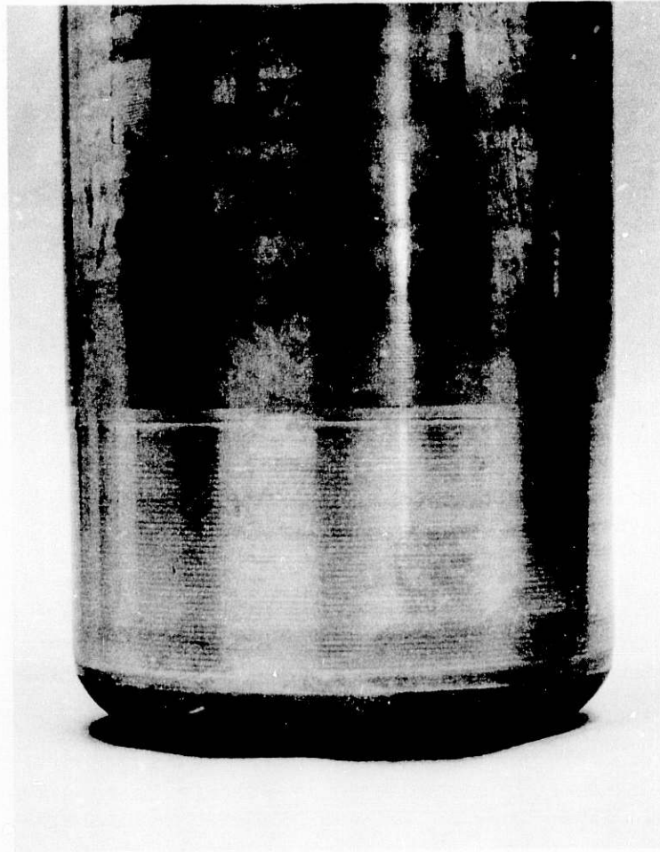
Fig. 15. Electrochemically Ground Sintered Tungsten Crucible. The machining feed lines are an indication of mechanical rather than electrochemical machining.
