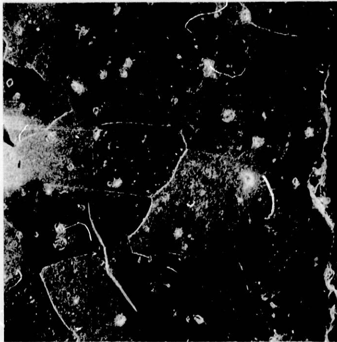
Fig. 2. SEM Micrograph of Polished Cross Section of Plasma-sprayed and Nickel-treated Tungsten after Exposure to Zn and \text{CaCl}_2\text{-KCl} at 800^\circ\text{C} for 120 h. Magnification, 1200X. ANL Neg. No. 306-79-690
