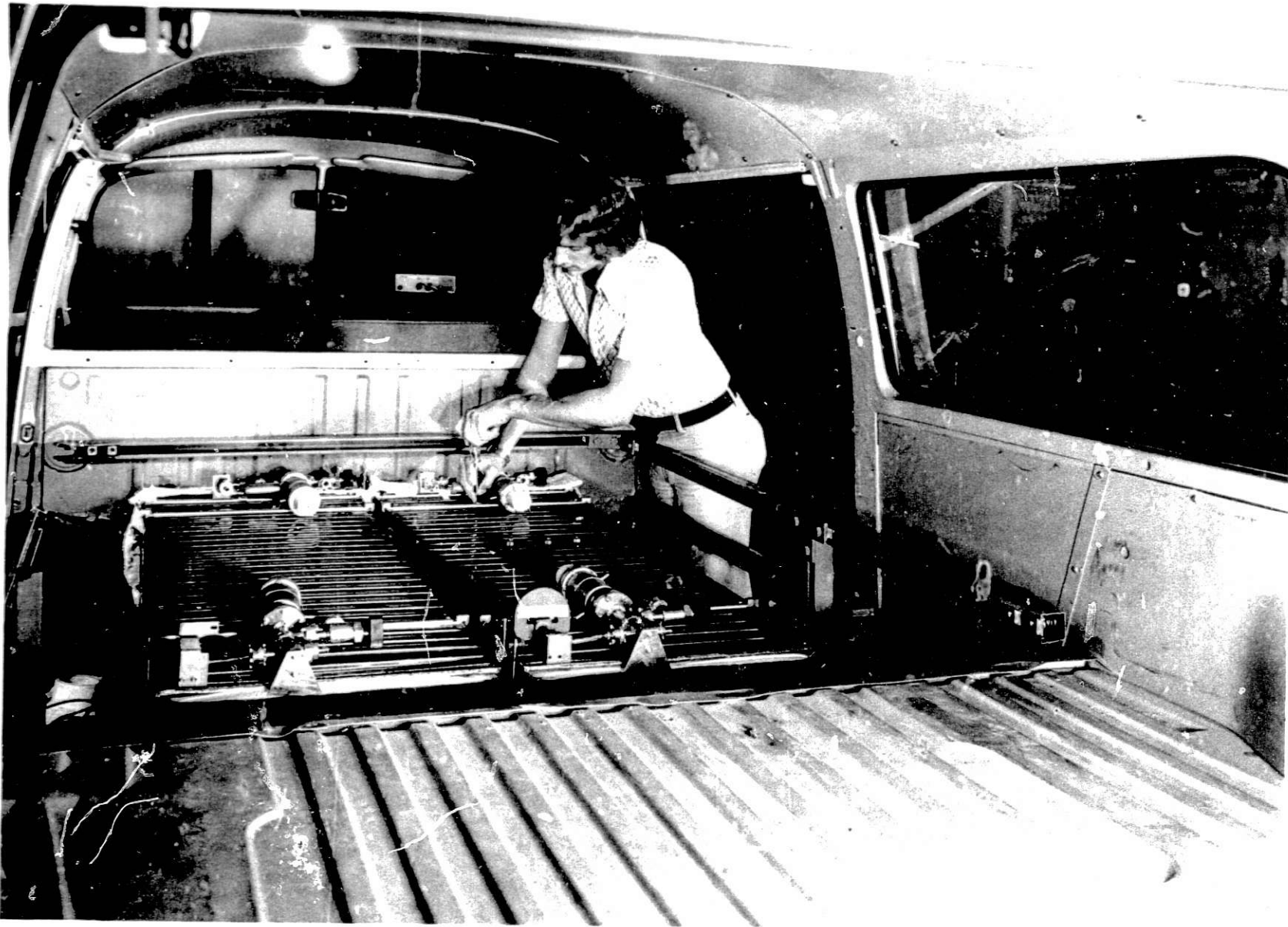
Fig. III-1. Modules D-001 and D-002 in Electric Van
