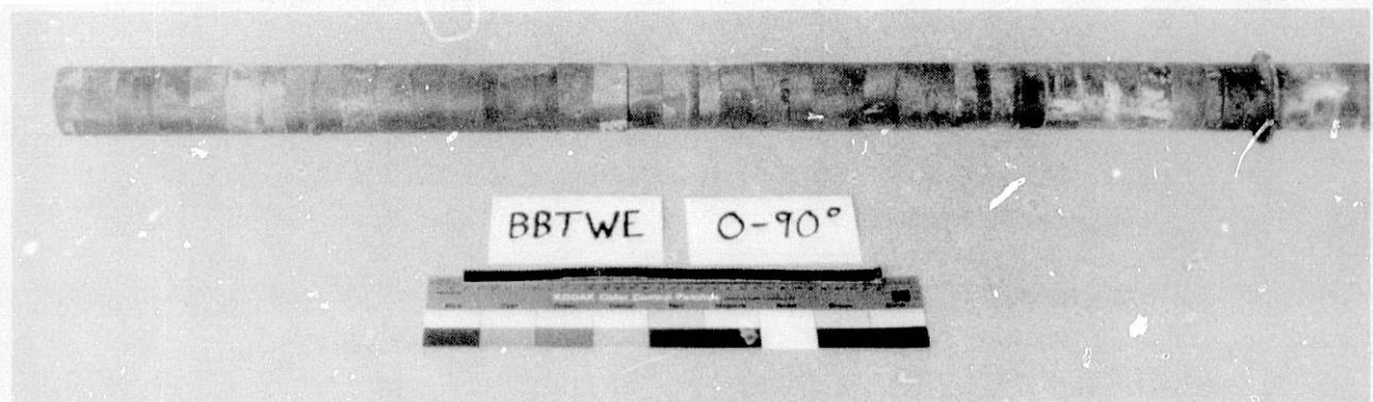
Fig. VI-10. Cooled Probe BBTWE (FW) at 1000 h
