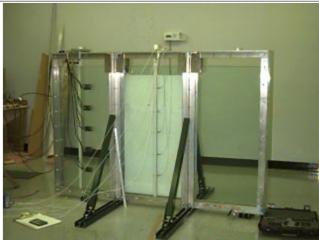
Figure 6. Water-Filled, Clean Tank Cell Showing the Test Set-up with a Five Acoustic Source Array and Five Pressure Transducers
