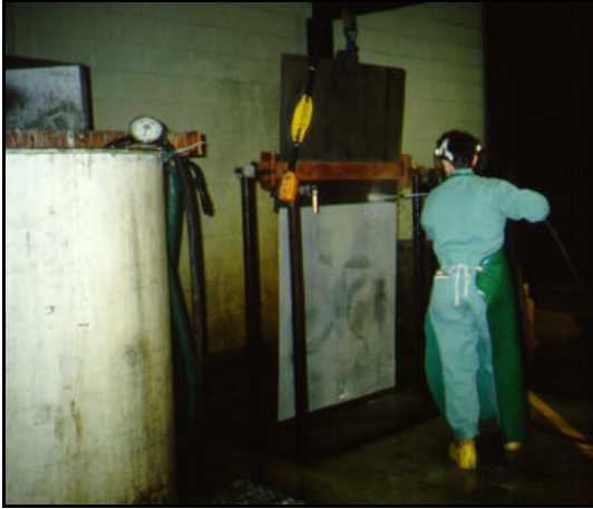
Photo 4 - Washing the sheet after descaling
