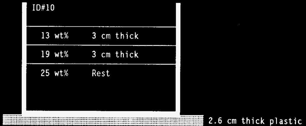
Figure 10. Layered 13, 19 and 25 wt% Standard
