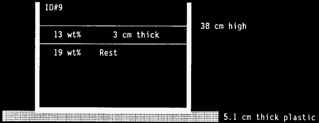
Figure 9. Layered 13 and 19 wt% Standard
