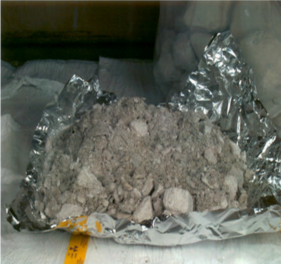
Figure 5: The asbestos portion of pipe lagging from Yankee Atomic was coned and quartered to provide test samples.
