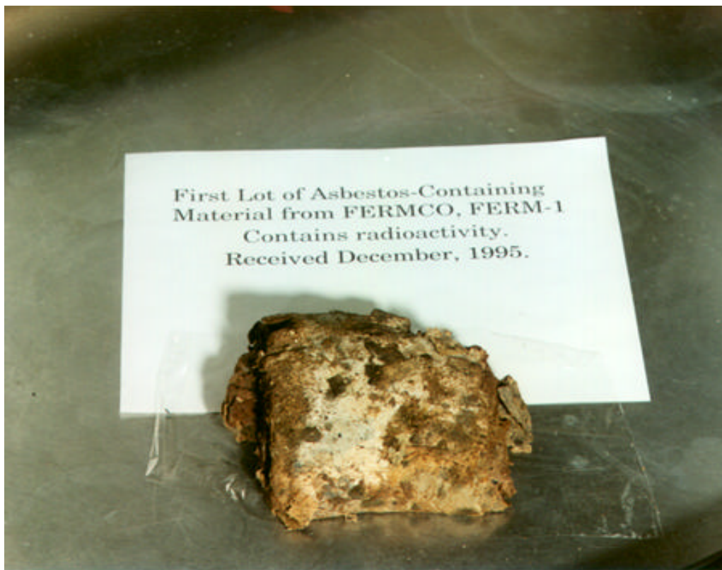
Figure 3: Asbestos pipe lagging samples from FERMCO contained discrete layers of asbestos wrapped in tar paper and aluminum foil.
