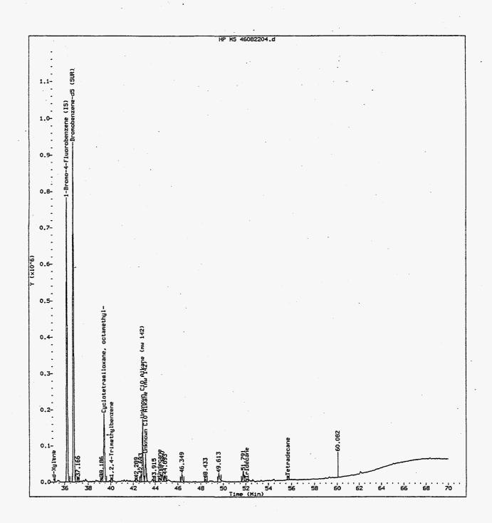
Figure E.1b Total Ion Chromatogram (36 - 70 min) for Hanford Waste Tank S-101 Triple Sorbent Trap Sample S6058-A13-1024 Collected on 6/6/96
