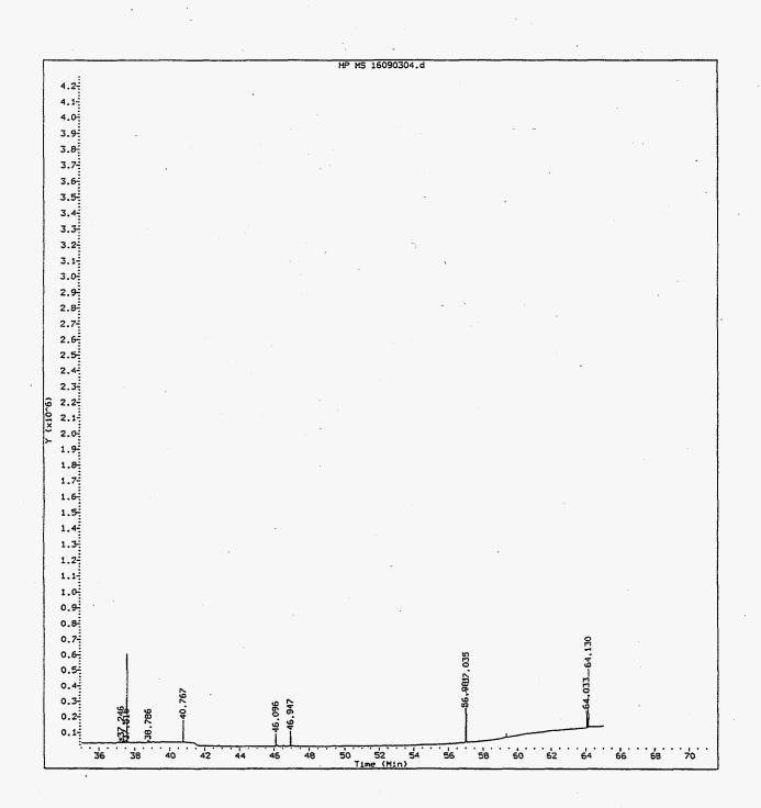
Figure D.1b Total Ion Chromatogram (36 - 70 min) for Hanford Waste Tank S-101 SUMMA<sup>™</sup> Canister Sample S6058-A05-311 Collected on 6/6/96
