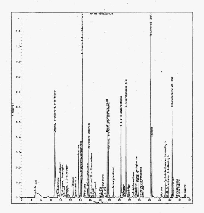
Figure E.1a Total Ion Chromatogram (2 - 36 min) for Hanford Waste Tank S-101 Triple Sorbent Trap Sample S6058-A13-1024 Collected on 6/6/96
