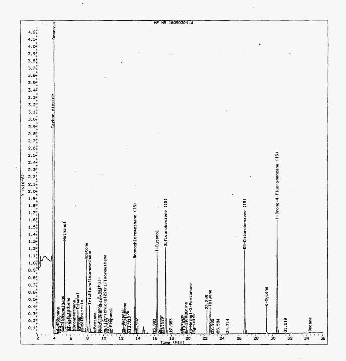
Figure D.1a Total Ion Chromatogram (2 - 36 min) for Hanford Waste Tank S-101 SUMMA<sup>™</sup> Canister Sample S6058-A05-311 Collected on 6/6/96
