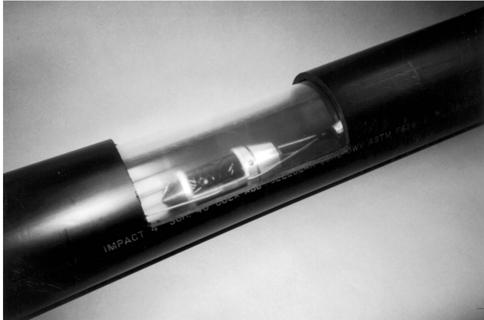
Figure 3. Cut-away view of a Pipe Explorer™ beta/gamma detector deploying through a pipe.
