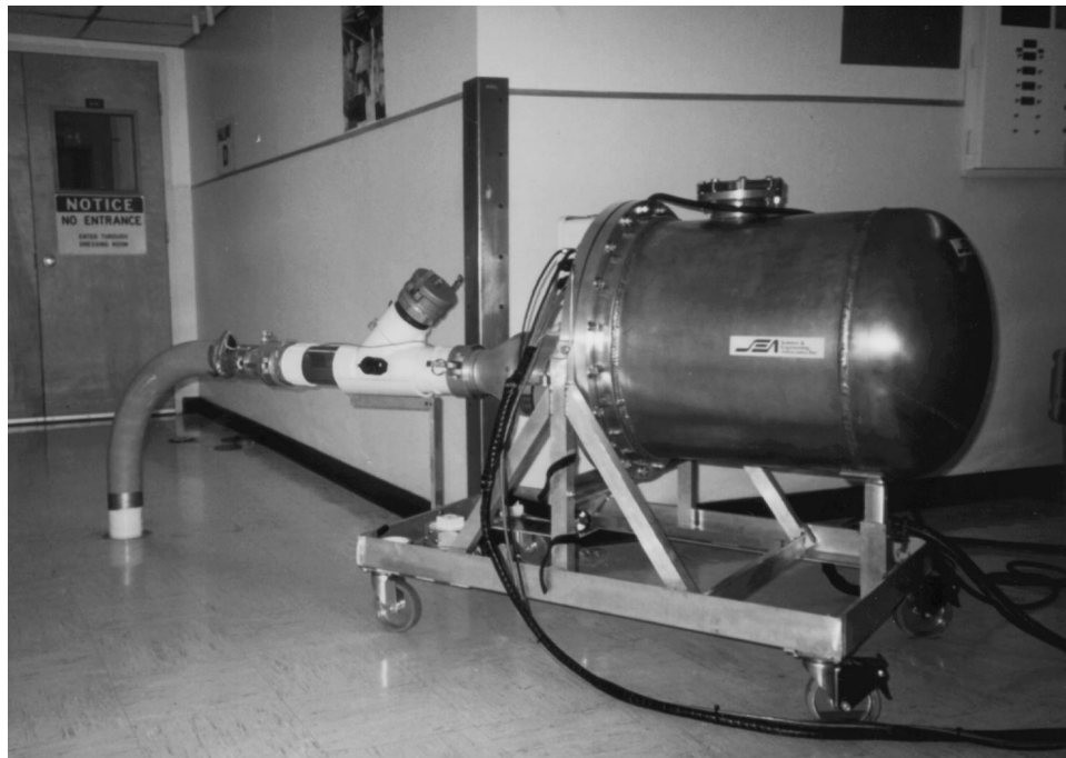
Figure 4. Photo of the SEA Pipe Explorer™ system in use at a DOE site.
