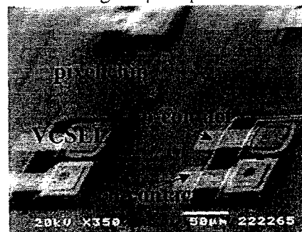
Fig. 7. SEM Photomicrograph of VCSEL's top-contacts bonded to a GaAs chip
