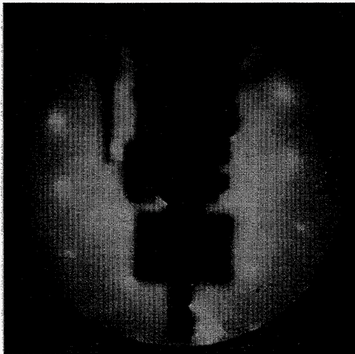
Figure 8.1 A LEED pattern corresponding to (2x2) overlayer at 98 eV. The (2x2) pattern was formed at 5 \times 10^{-5} torr of CO partial pressure. The LEED pattern shows no change for at least 30 minutes, then the back ground intensities start to increase.
