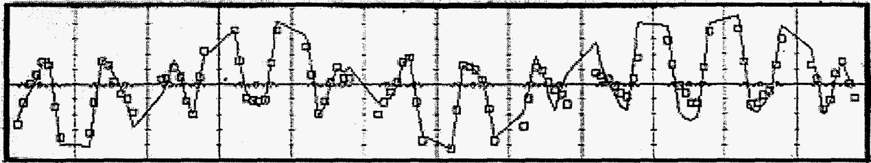
Figure 2. Horizontal closed-orbit distortion around the entire storage ring ( \pm 200\mu full scale) as measured on 9/12/96 (open symbols) and simulated by TRACY V (continuous line), assuming a progressive girder deformation of up to 31\mu .
