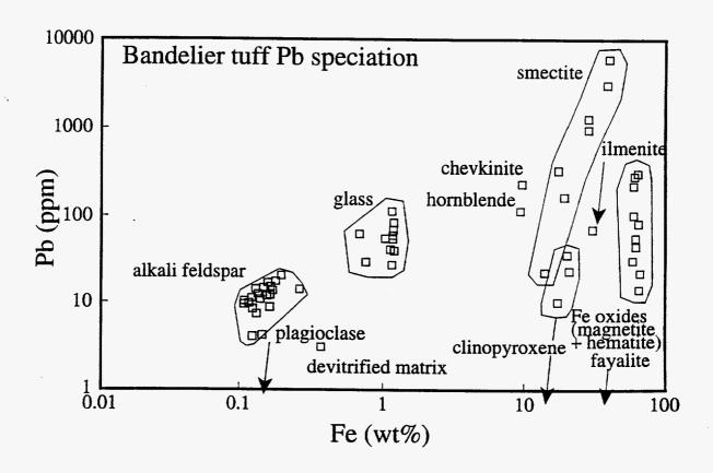
Figure 1. Lead (ppm) determined by PIXE versus Fe (wt.%) determined by electron microprobe analysis for minerals, glass and matrix for the Tshirege Member of the Bandelier tuff. Arrows indicate that some mineral grains have Pb concentrations below PIXE detection limits.
