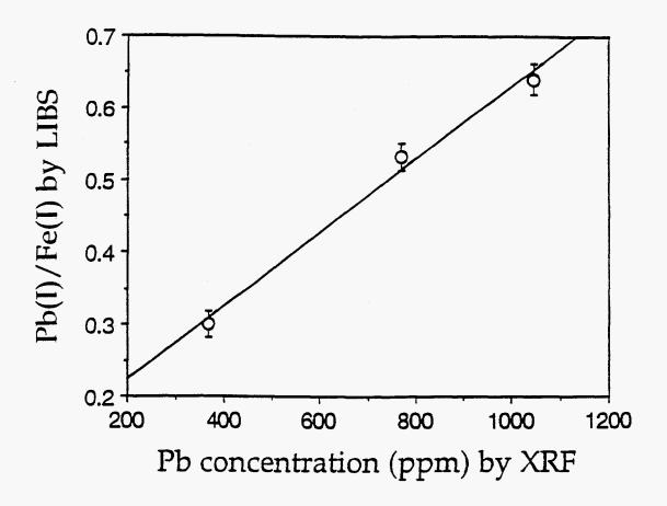
Figure 4. Working curve (Pb determined by LIBS versus Pb determined by XRF) for LIBS analysis of Pb in soils. Note excellent linear correlation between XRF results and LIBS results.
