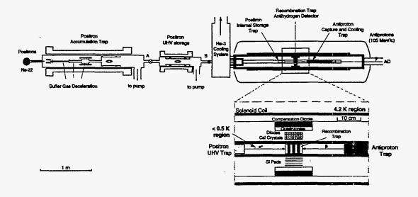
Figure 1. Overview of the ATHENA apparatus showing the superconducting solenoid with the antiproton capture trap, the positron storage trap, and the recombination trap surrounded by the magnetic gradient trap.
