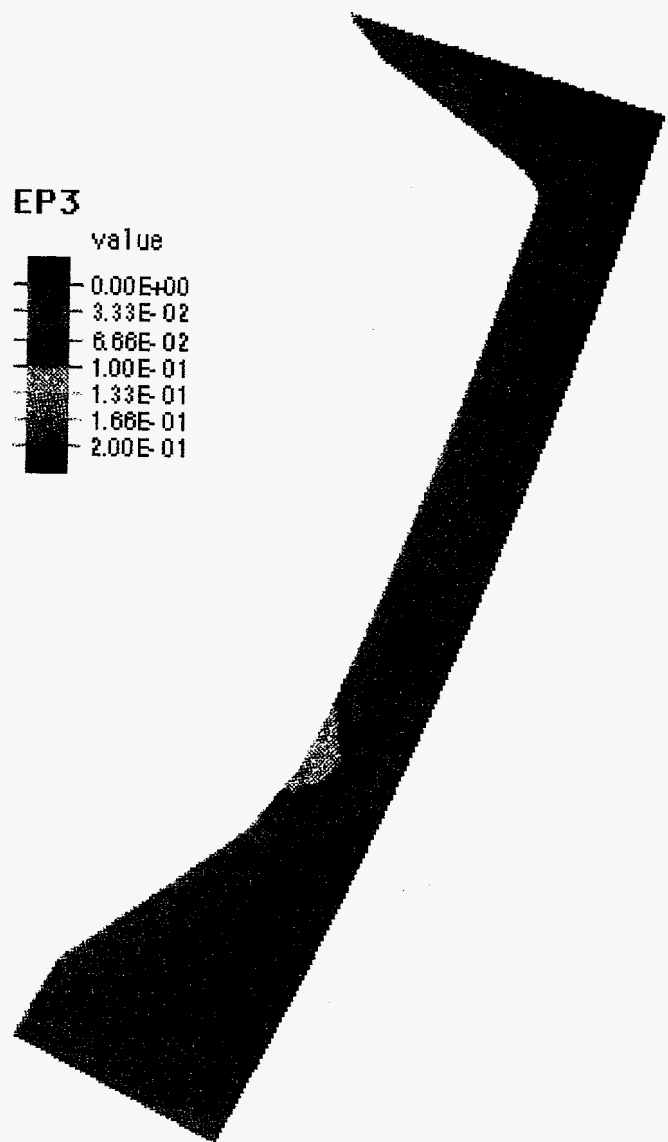
Figure 4.12. Map of maximum principal strain distribution.
