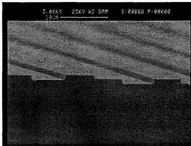
Figure 2. A scanning electron micrograph of an end view of a portion of the HF element.
