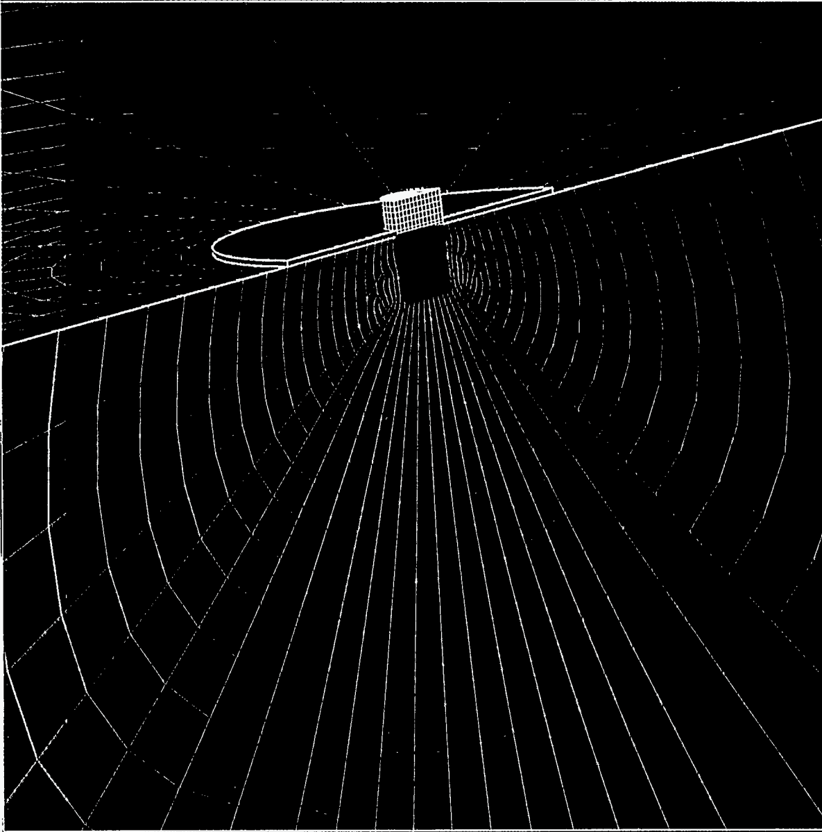
Figure 5.1 Mesh for the flat plate problem.
