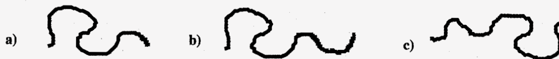
Figure IV.18 Illustration of relative block sizes for adsorbed copolymers using a) pure methanol, b) 80/20 by weight methanol/water solution, 0.002 wt fraction, c) 80/20 by weight methanol/water solution, 0.062 wt fraction. Red = imidazole block, Blue = amine block
