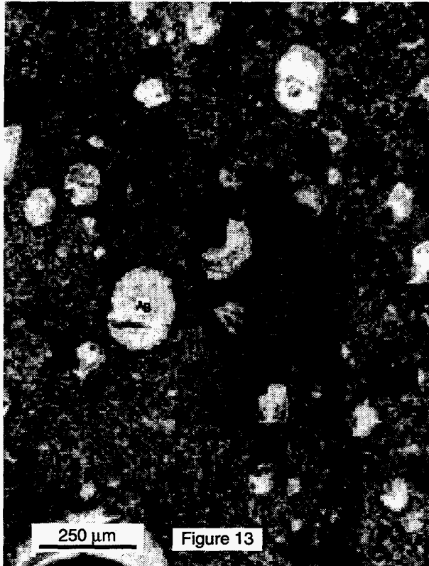
Figure 13: Microstructure in 1-g processed, unannealed 29 wt % Ag/Y123 composite processed at a heating rate of 100 °C/s.
