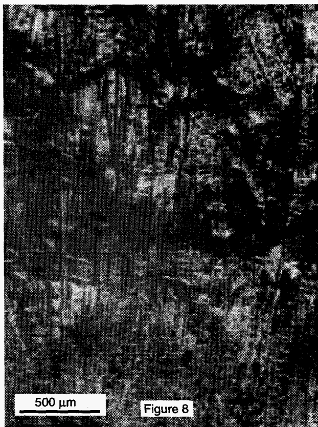
Figure 8: Microstructure in 0g processed, melt-textured, Y123 with vertical orientation in direction of zone movement.
