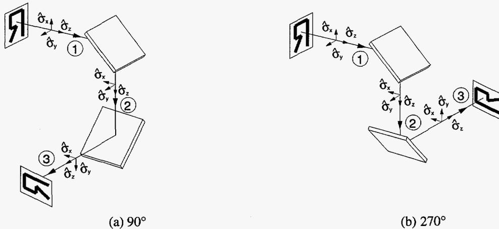
Figure 2.2.  $\pm 90^\circ$  out of plane reflections.
