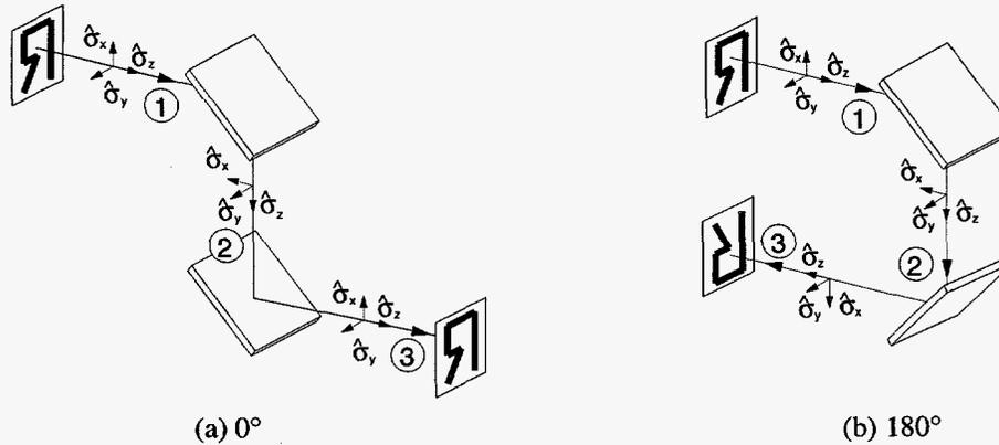
Figure 2.1. In-plane two mirror reflections.
