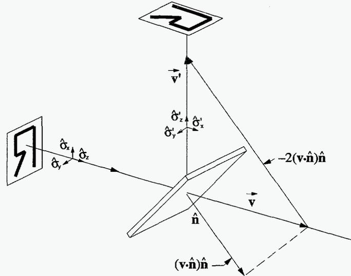
**Figure 4.1.** There is no pattern rotation about the output ray axis in a single mirror reflection.
