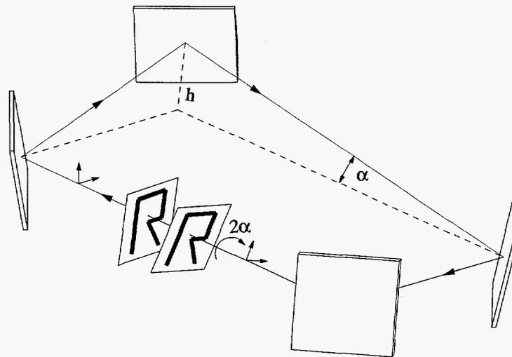
**Figure 4.3.** Pattern rotation in a four mirror ring.
