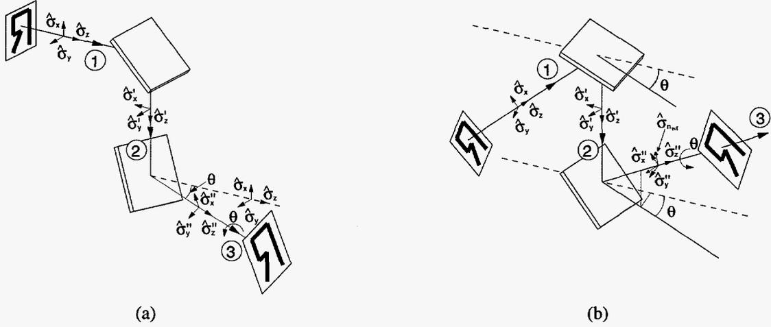
**Figure 4.2.** Layouts for two mirror pattern rotation problems.
