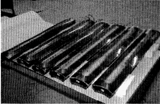
Figure 1. Sextupole coils after vacuum impregnation prior to assembly.
