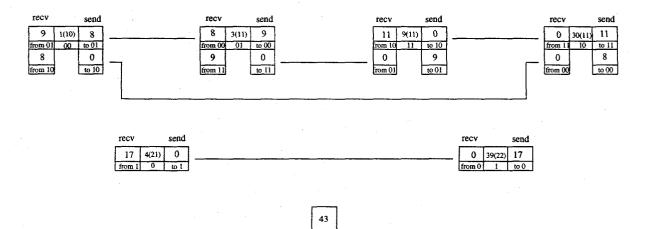
Here the number in the center of each node is the accumulated load, the number behind that in parenthesis is the desired load. The columns on the left and on the right of each node contain the amount of load that has to be received or sent along the specified edge in the hypercube.
