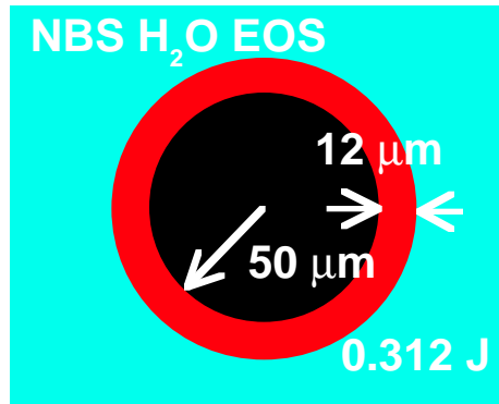
Fig. 14. Geometry used for the ERM to compare to the 2-D LATIS simulations.
