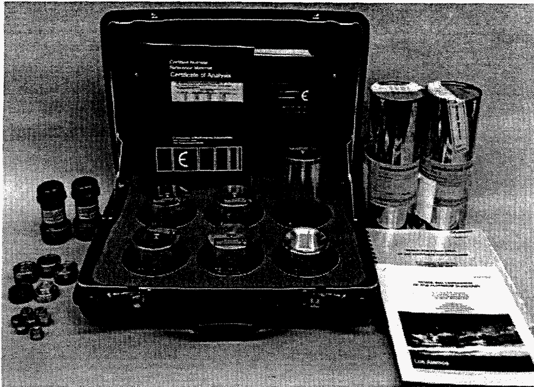
Figure 3. Assembly of many of the NDA calibration standards discussed in this paper. In the carrying case are the Geel enrichment standards (NBL-SRM-969). To the left of the carrying case, in the foreground, are the PIDIE Pu isotopic standards; in the left background are the CBNM Pu isotopic standards. To the right of the carrying case are two of the SGS can standards containing plutonium oxide.
