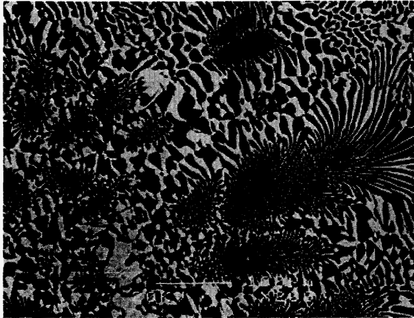
Fig. 1. Typical microstructure of as-cast SS-15Zr alloy. The dark phase is \alpha -SS, the bright phase Zr(Fe,Cr,Ni)_{2+x} .
