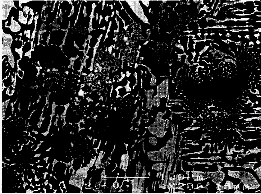
Fig. 2a. Microstructure of SS-15Zr alloy annealed for 2h at 1275°C. The dark phase is \alpha -SS, the bright phase is Zr(Fe,Cr,Ni)_{2+x} , and the gray phase is (Fe,Cr,Ni)_{23}Zr_6 .
