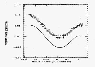
Figure 4: Experimental phase-phase transfer function obtained at the Jefferson Lab injector, and its synthesis using the Tschebyshev expansion (displaced for comparison).
