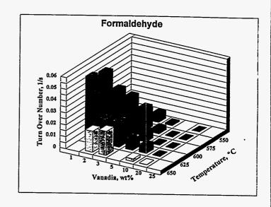
**FIGURE 3.** Turnover numbers of formaldehyde and methanol as functions of the reaction temperature and vanadia content of the  $V_2O_5/SiO_2$  xerogel catalysts. Reaction conditions are given in Table 1.
