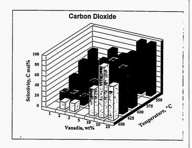
**FIGURE 1.** Selectivities of products as functions of the reaction temperature and vanadia content of the  $V_2O_5/SiO_2$  xerogel catalysts. Reaction conditions are given in Table 1.
